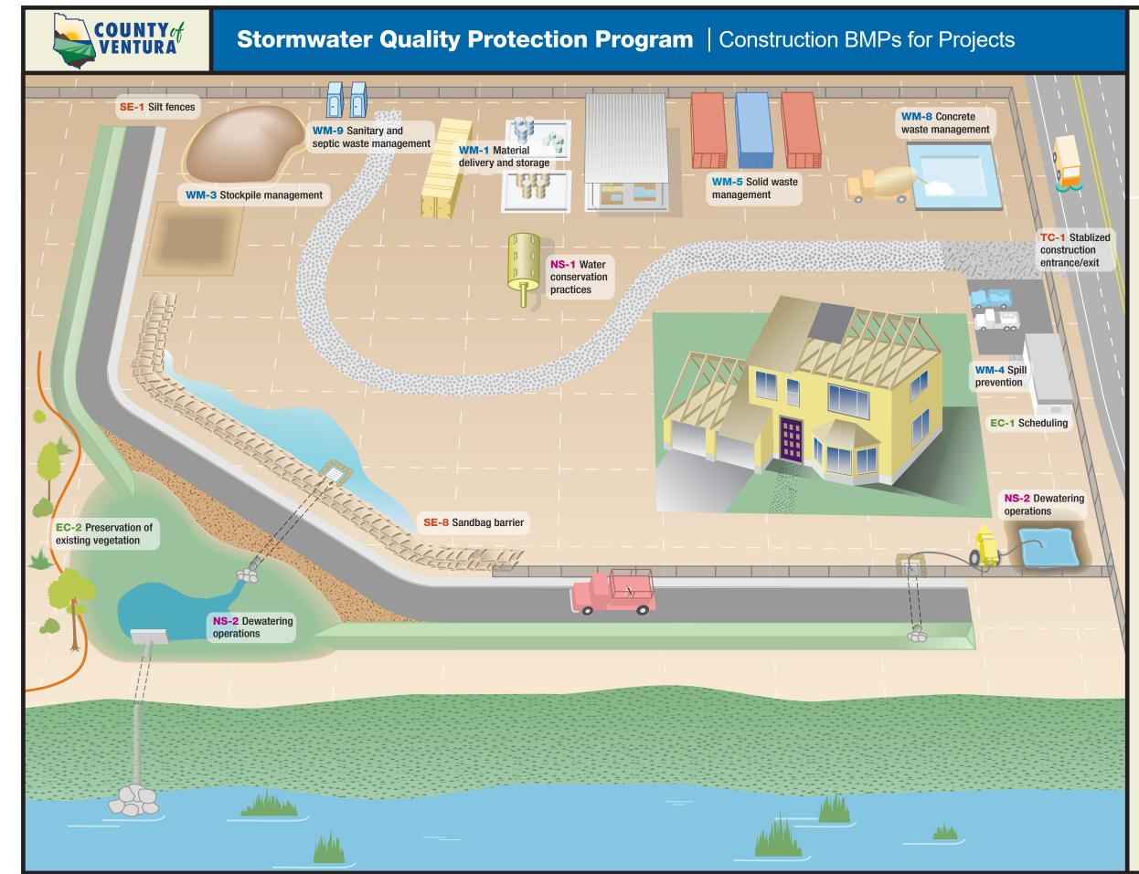
Stormwater runoff in the County drains directly into local creeks and into the ocean. Implementing Best Management Practices (BMPs) to keep construction site runoff clean is an important part of the County's program. This brochure describes BMPs that must be implemented for construction projects.
